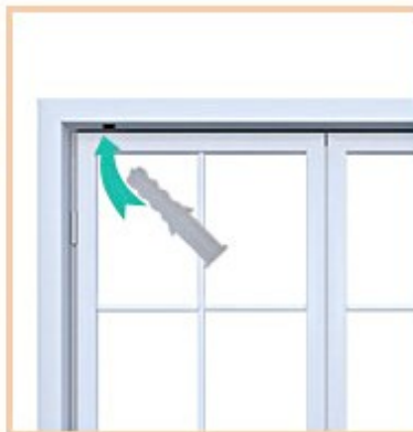
03. Plug the expansion screw into holes
